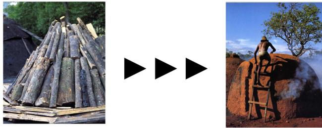
Figure 4: Charcoal production is controlled combustion of wood under controlled air supply.
