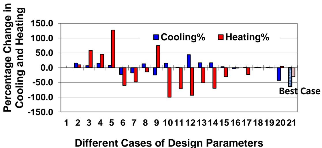
Figure 8: Percentage change in the annual cooling and heating loads for changes in various design parameter of the house to maintain optimum indoor thermal comfort.
