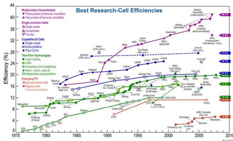
Figure 13: Best conversion efficiency of various types of experimental solar cells.
