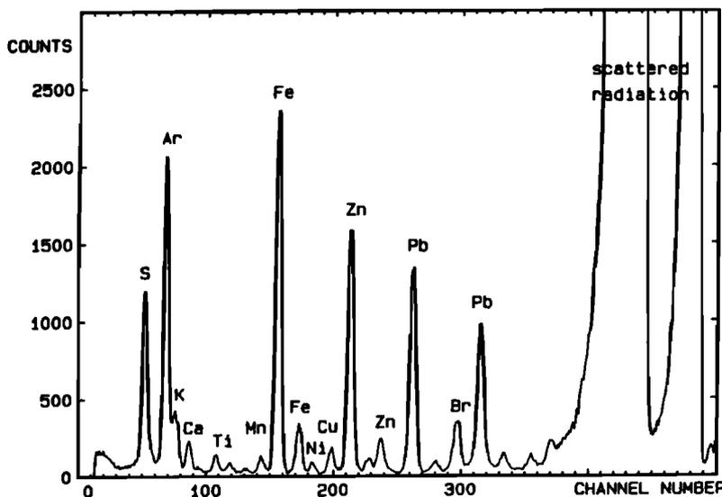
**Figure 2.** A typical aerosol spectrum of coarse and fine particles from an EDXRF analysis. Characteristic lines, which are marked by their respective elements, and the background under the characteristic lines are shown. With the exception of lead, for which L- $\alpha$  and L- $\beta$  radiation are displayed, K x rays are displayed for all elements. The channel number is linearly proportional to the x-ray energy.
